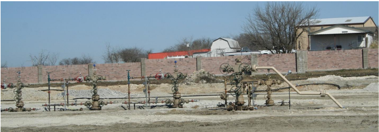
Figure 13. Photograph shows a saline water disposal (SWD) well co-located with three hydrofractured wells. At this site, the saline water was being injected into the Ellenburger formation that is below the shale-gas formation layer.
