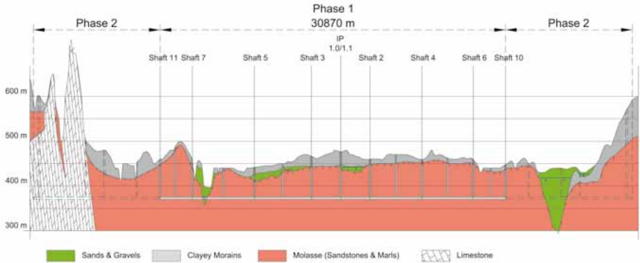
Figure 5.15 Tunnel geology of the CERN region.
