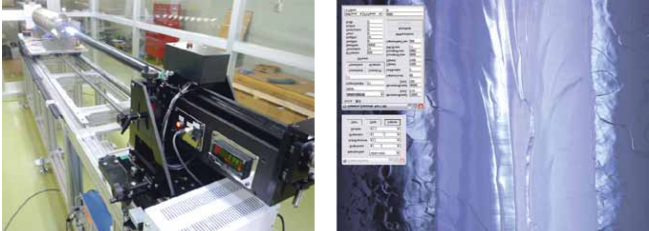
Figure 2.4 Left: Kyoto-KEK optical inspection camera system. Right: an example of automated image capture software.
