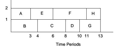
Figure 3. Schedule and Resource Loading Associated with the Sequence [BAECFHDG].
