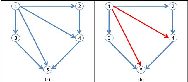
Figure 12. Transportation Network (a) nominal state and (b) disrupted state. Red indicates links have no capacity.
