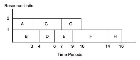
Figure 2. Schedule and Resource Loading Associated with the Sequence [A B C D E F G H].
