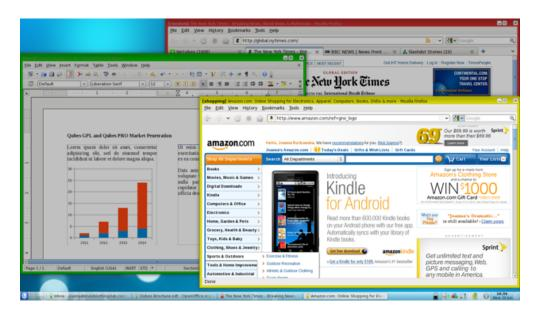
Figure 1: **Security levels in Qubes OS**: Qubes OS creates VMs with different security levels. Red is least trusted: Browse any website, but don't enter any secure data. Yellow is somewhat trusted: Browse only trusted websites, and enter limited secure data. Green is most trusted: Avoid nearly all web use, enter any secure data.
