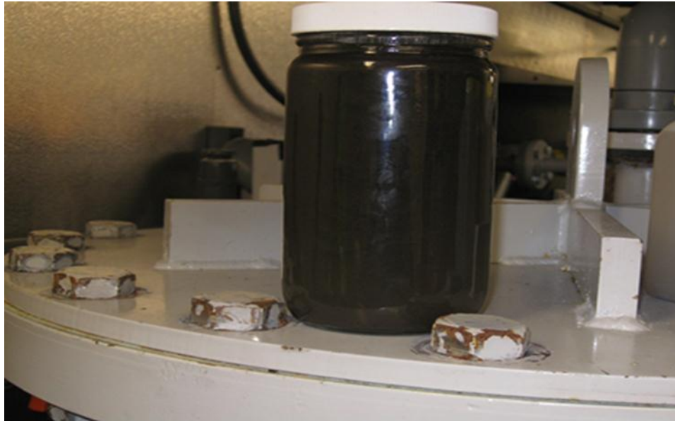
Figure 14: Oil/Polymer Mixture Treated by MTU
