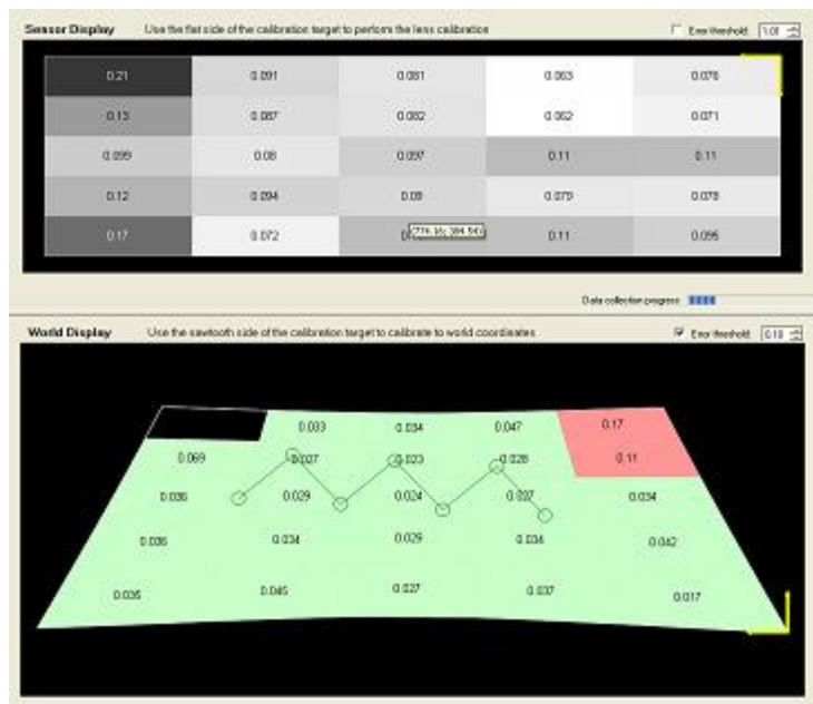
Figure 2 Camera and laser distortion correction results
