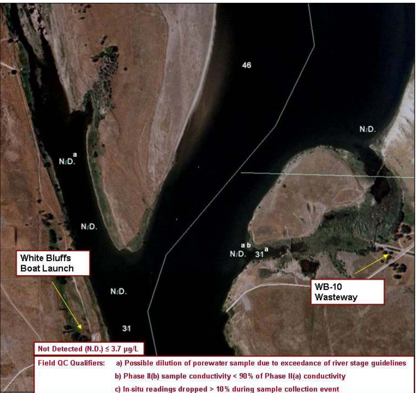
Figure 3-41. Pore Water Hexavalent Chromium ( \mu\text{g/L} ) Levels Measured During Phase II(b) Near the 100-H Area (Sheet 2 of 2).
