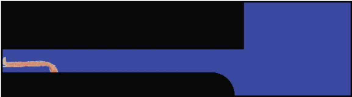
Figure 8. Plot of electron temperatures near Bernard Long insulator, computed by LSP and imported to ALEGRA-HEDP.
