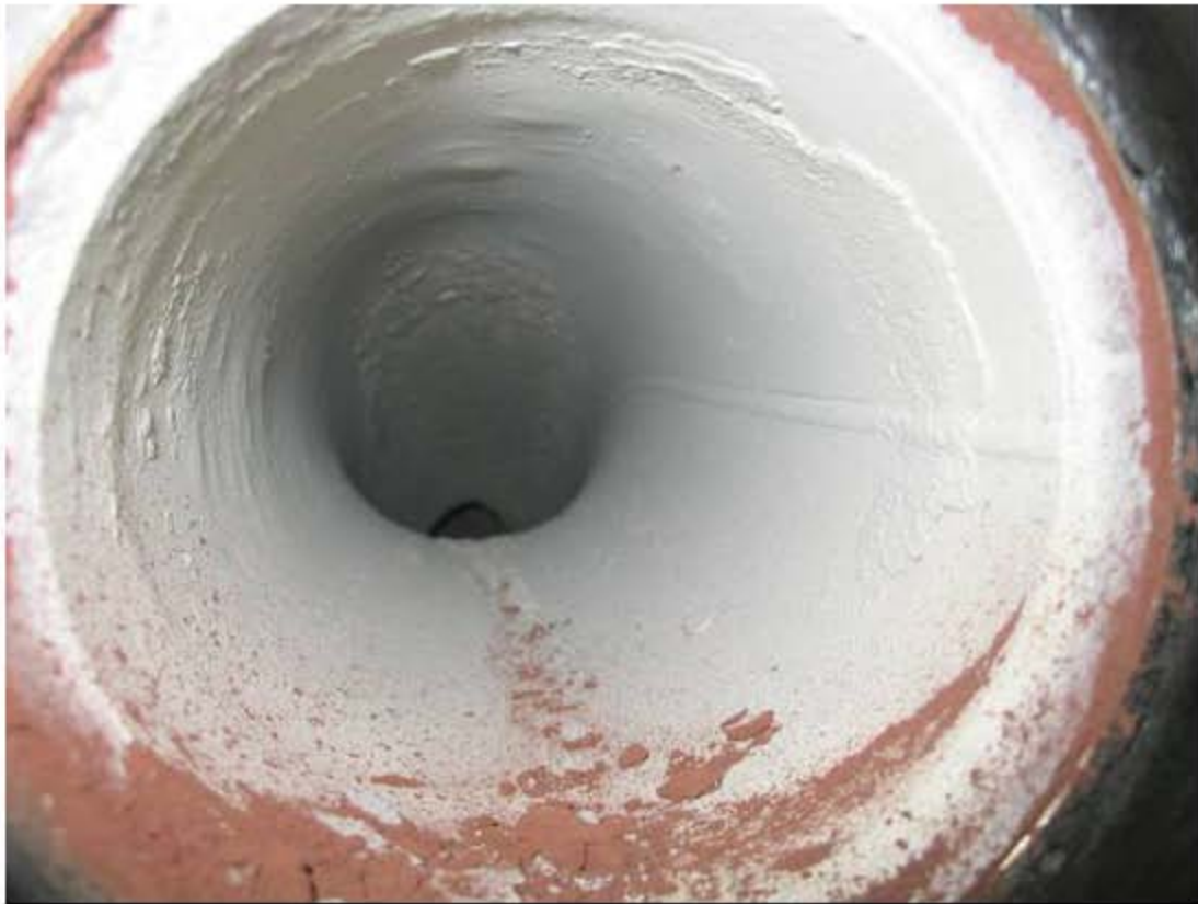
Figure 4.75. Inlet of transition line section in between bellows and SBS inlet after HLW Turnover Test following the MACT tests [41].
