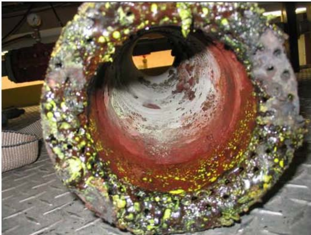
Figure 4.63. Film cooler inlet after HLW Turnover Test following the MACT tests [41].
