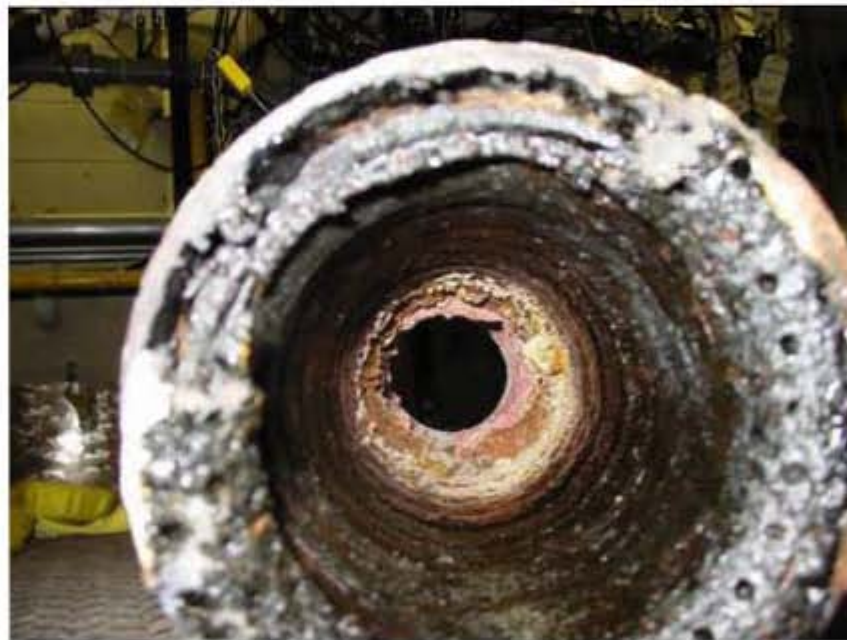
Figure 4.10. View of bottom of the removed film cooler (pre-cleaning) after tests with LAW Sub-Envelope Al simulants [14].
