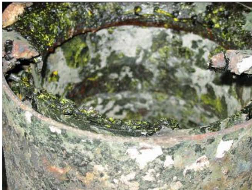
Figure 4.17. View of louvers of the film cooler (pre-cleaning) after tests with LAW Sub-Envelope A1 simulants [14].
