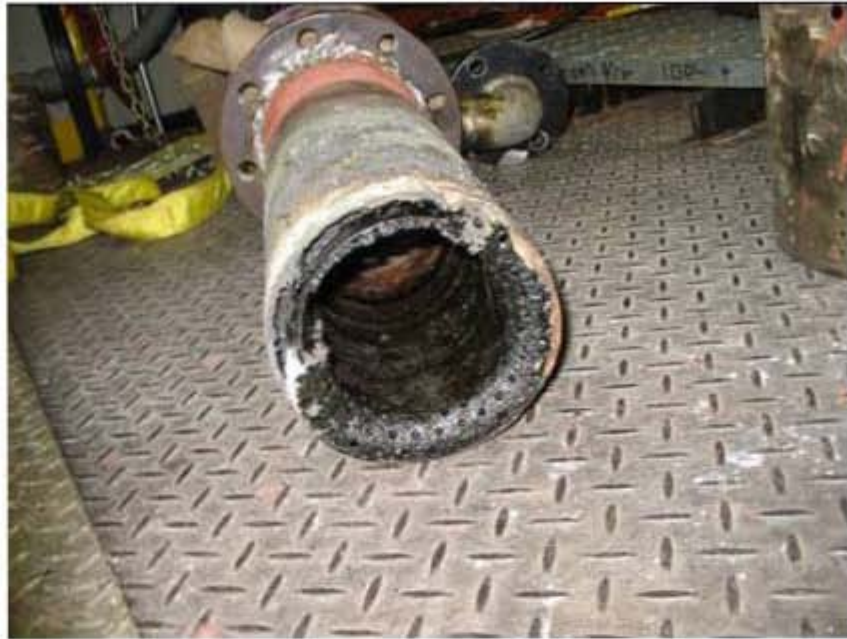
Figure 4.10. View of bottom of the removed film cooler (pre-cleaning) after tests with LAW Sub-Envelope Al simulants [14].
