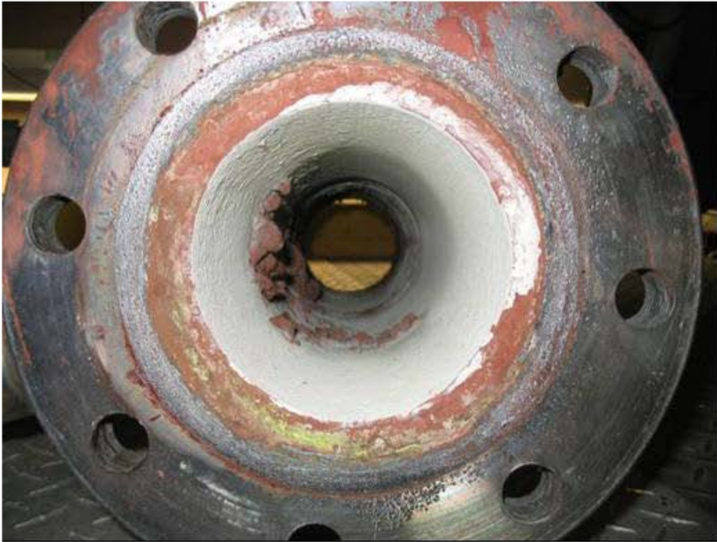
Figure 4.66. Film cooler outlet after HLW Turnover Test following the MACT tests [41].
