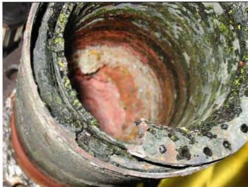
Figure 4.12. View of fractured bottom ring of the film cooler (pre-cleaning) after tests with LAW Sub-Envelope Al simulants [14].
