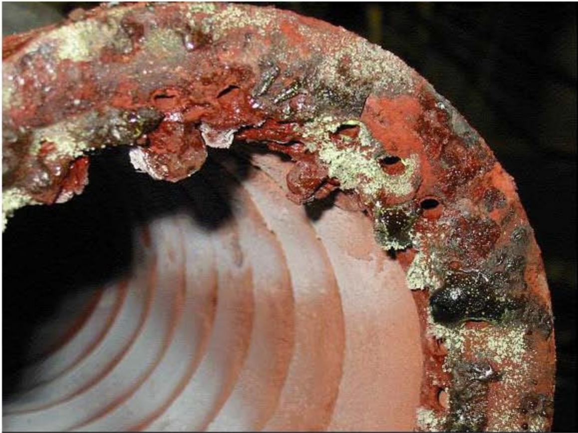
Figure 4.28. Film cooler inlet close-up after tests with HLW C-104/AY-101 simulants [28].
