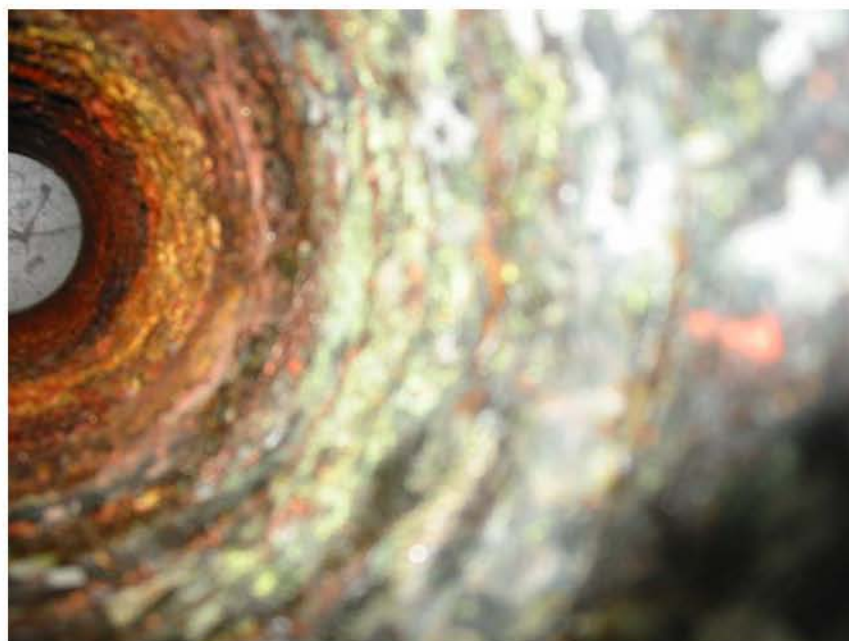
Figure 4.23. Close-up view of exit end of the film cooler (post cleaning) after tests with LAW Sub-Envelope A1 simulants.
