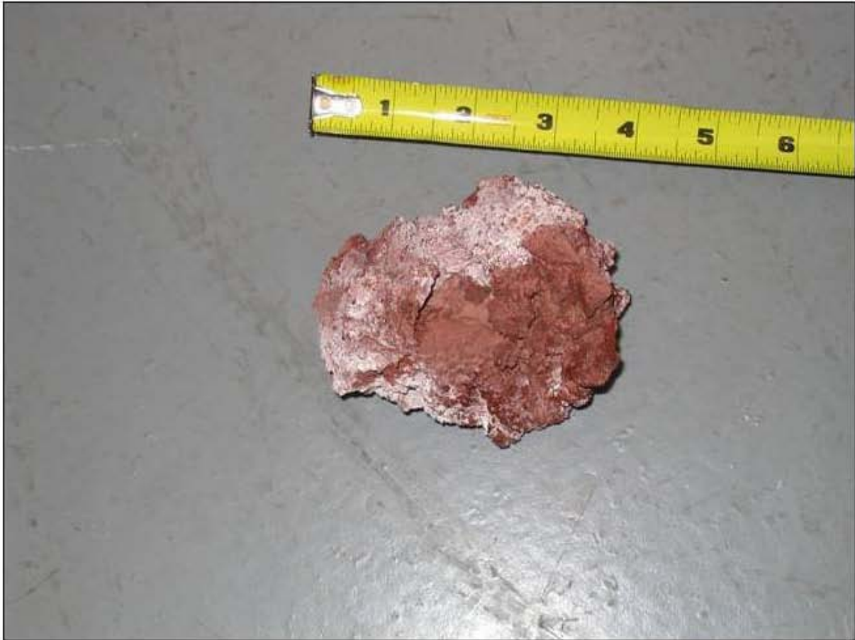
Figure 4.43.a. View of large debris removed from transition line bellows inlet during Configuration Test 3 [30].
