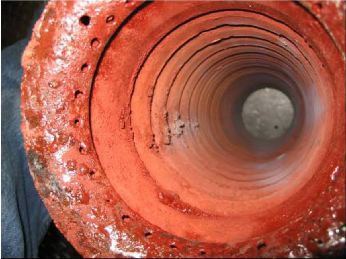
Figure 4.44. Close-up of clogged perforation of film cooler inlet after Configuration Test 3 [30].
