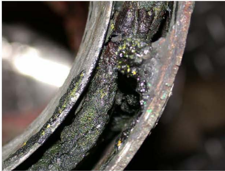
Figure 4.16. View of glass and weld beneath the failed region of film cooler (pre-cleaning) after tests with LAW Sub-Envelope A1 simulants [14].
