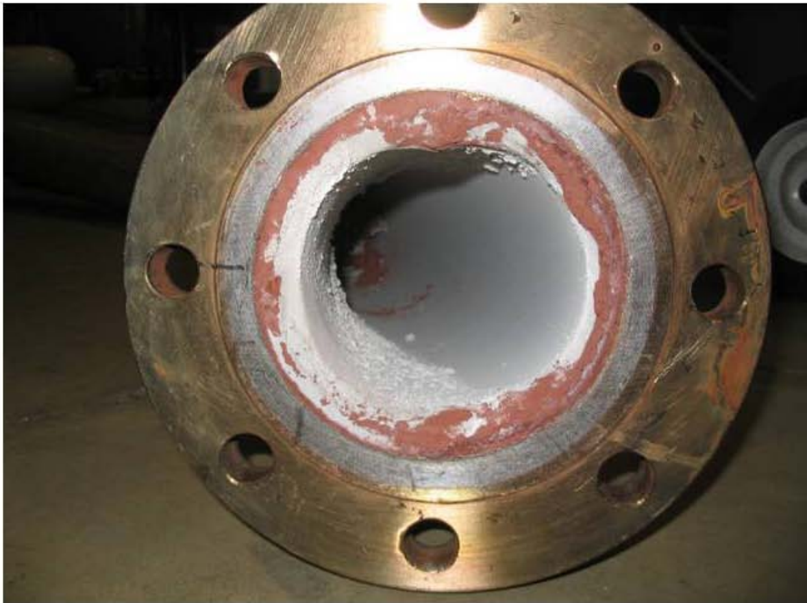
Figure 4.48. Transition line section #2 inlet after Configuration Test 10 [30].
