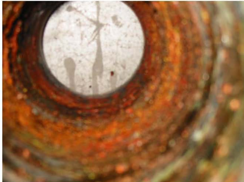
Figure 4.22. View of exit end of the film cooler (post cleaning) after tests with LAW Sub-Envelope A1 simulants.
