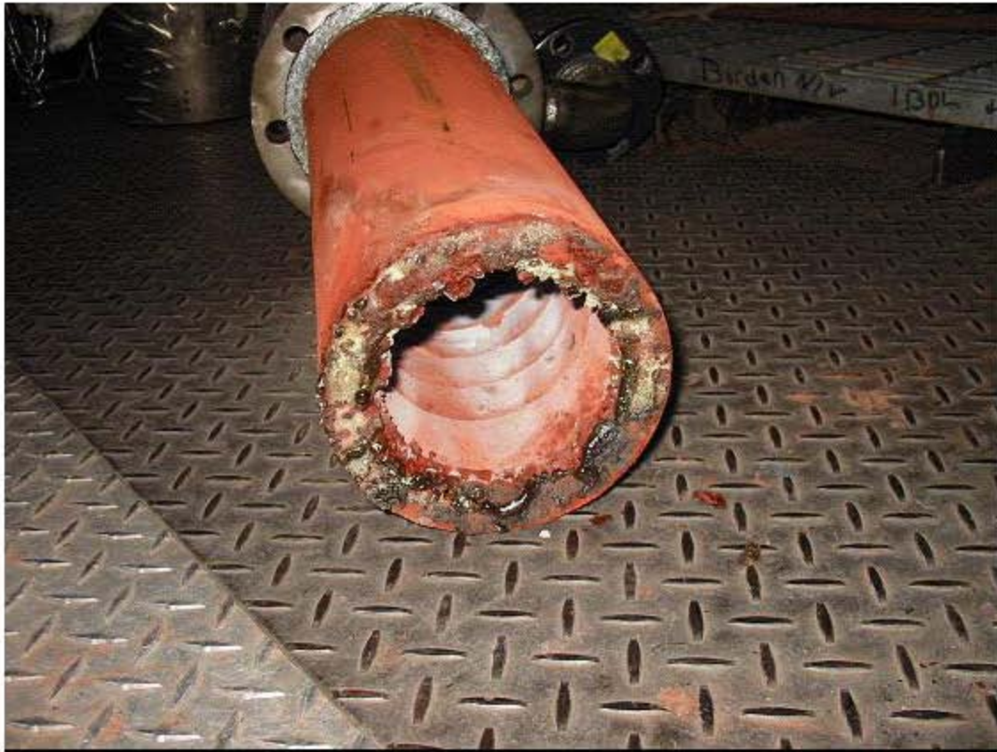
Figure 4.27. Film cooler inlet after tests with HLW C-104/AY-101 simulants [28].
