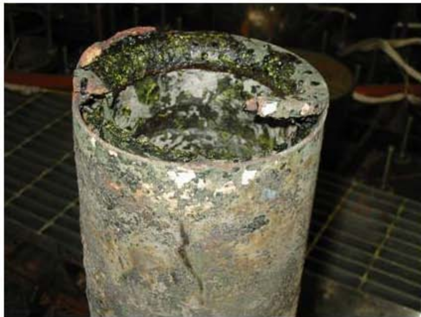
Figure 4.18. View of louvers of the film cooler (pre-cleaning) after tests with LAW Sub-Envelope A1 simulants [14].
