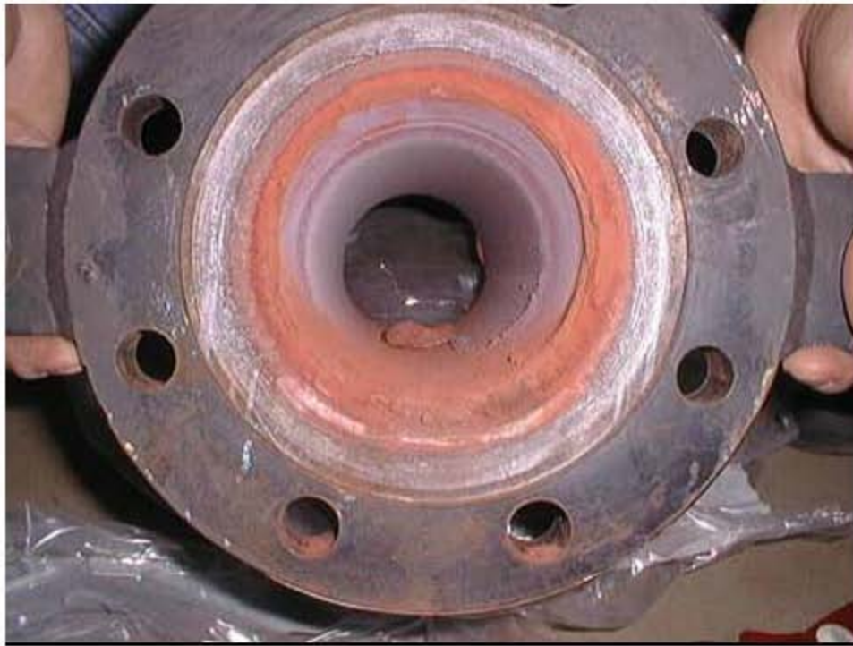
Figure 4.39. Transition line bellows inlet after Configuration Test 2 [30].
