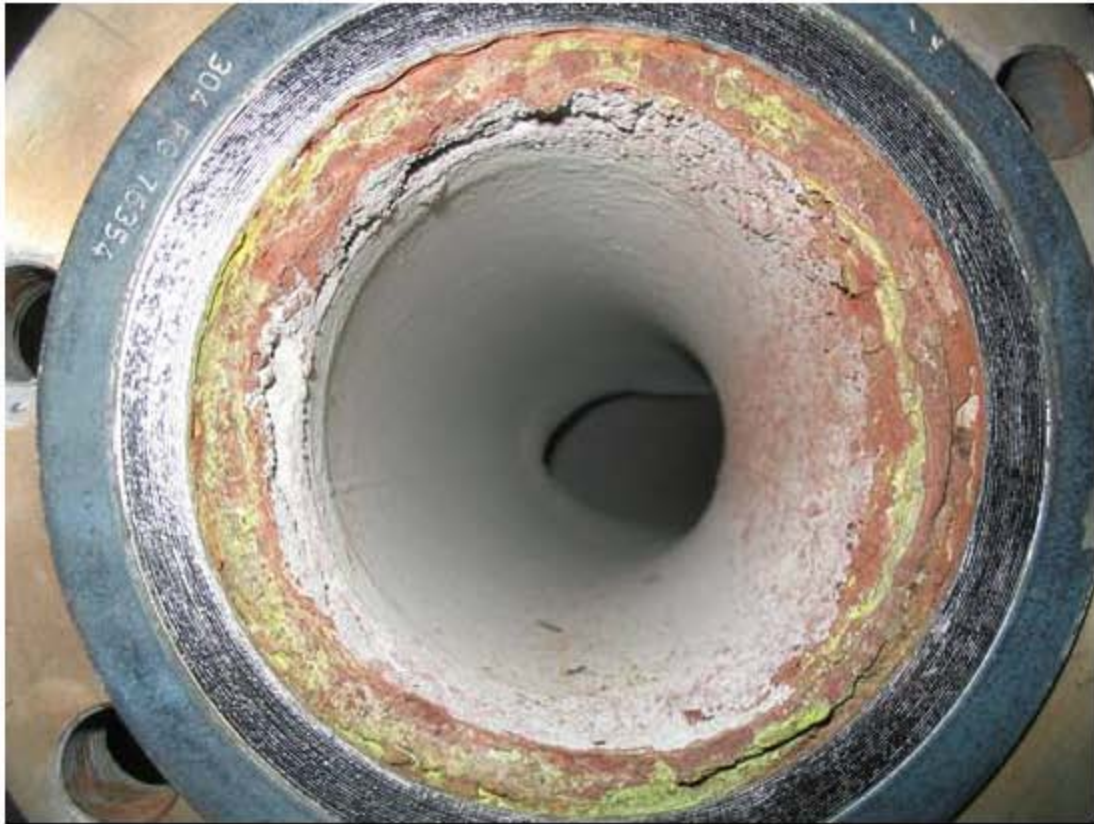
Figure 4.70. Transition line section #1 outlet after HLW Turnover Test following the MACT tests [41].
