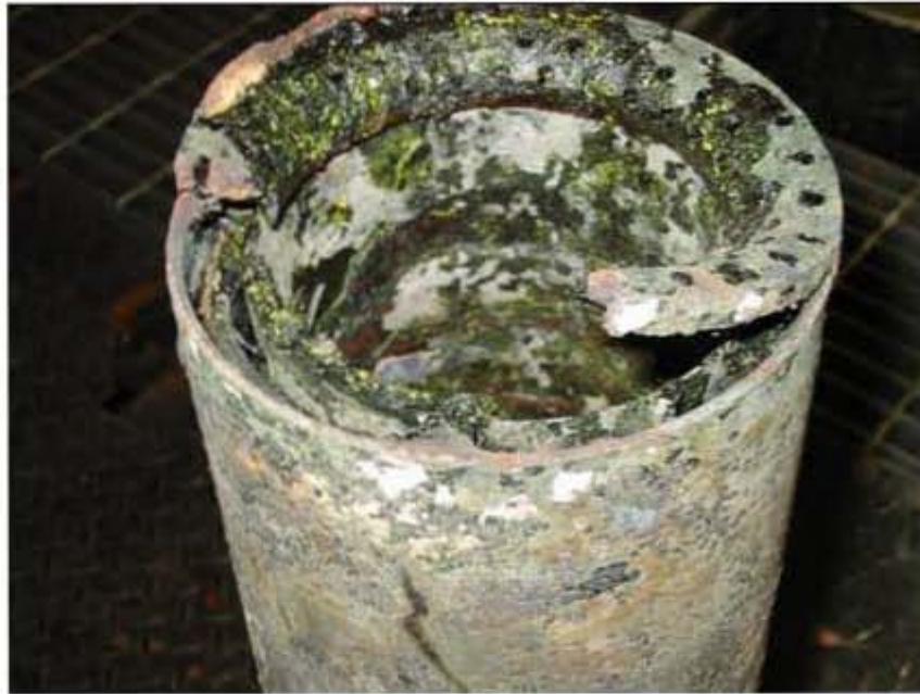
Figure 4.12. View of fractured bottom ring of the film cooler (pre-cleaning) after tests with LAW Sub-Envelope Al simulants [14].
