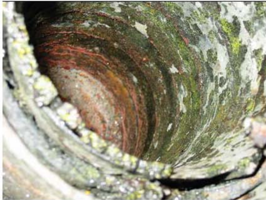
Figure 4.18. View of louvers of the film cooler (pre-cleaning) after tests with LAW Sub-Envelope A1 simulants [14].
