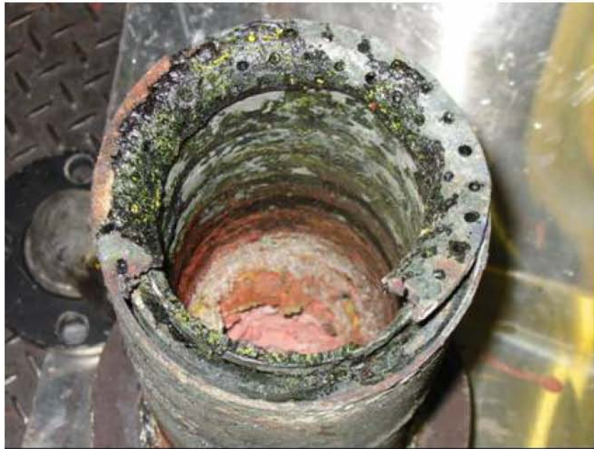
Figure 4.14. Another bottom view of the film cooler (pre-cleaning) after tests with LAW Sub-Envelope A1 simulants [14].
