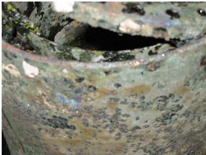
Figure 4.15. View of detachment of the film cooler bottom ring (pre-cleaning) after tests with LAW Sub-Envelope A1 simulants [14].
