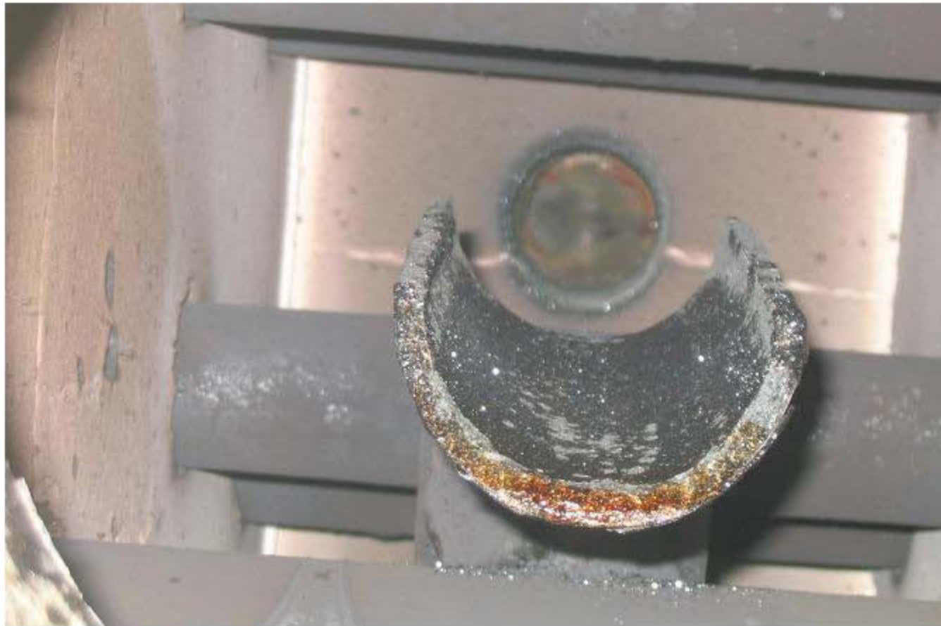
Figure 2.20. View of the inside of the DM1200 discharge chamber showing the fiberboard walls and the end of the discharge trough. View up through the discharge port on the bottom of the chamber.
