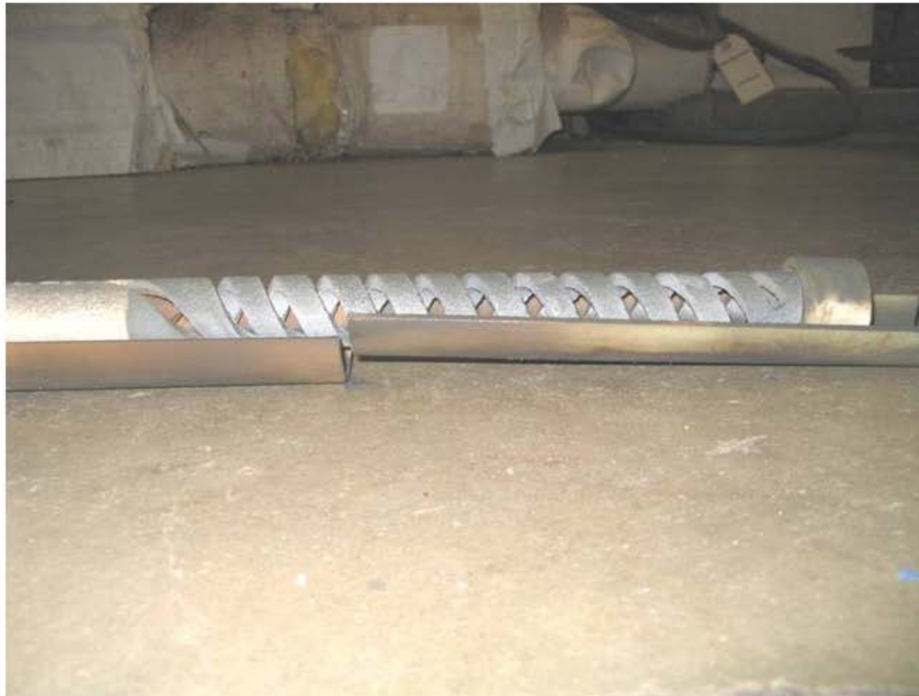
Figure 2.11. Typical discharge heater in the modified ceramic isolator. This assembly was installed in metal sheaths located in the discharge chamber.
