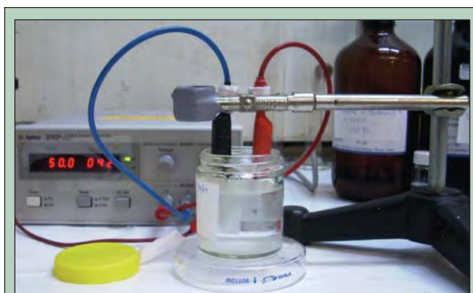
Figure 1. The anodization setup features a DC power supply, an electrolyte bath, and two electrical wires suspending two electrodes in the electrolyte bath. The black lead holds the Pt counter electrode, and the red one holds the zirconium foil to be anodized.
