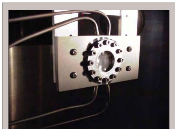
Figure 4. Photograph of flowing water target used in Jefferson Lab experiments.
