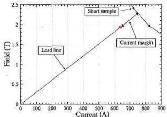
Fig. 8. Load line and expected short-sample limit.
