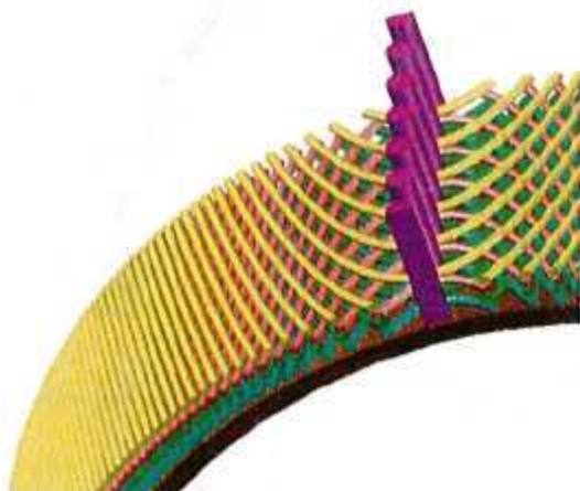
Fig. 3. View of layers wound around pins (poles).
