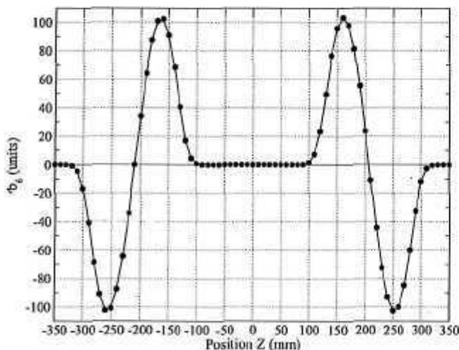
Fig. 6. Allowed harmonic  $b_0$  calculated at a radius of 17 mm corresponding to 45% of the bore radius.
