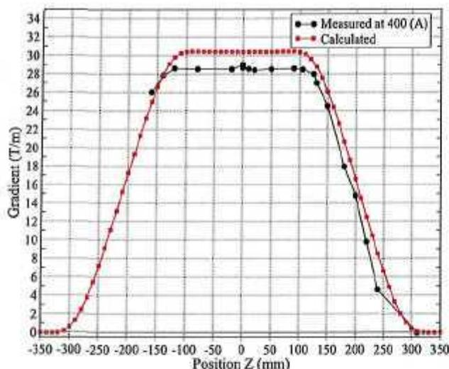
Fig. 9. Axial scan of measured and calculated gradient.
