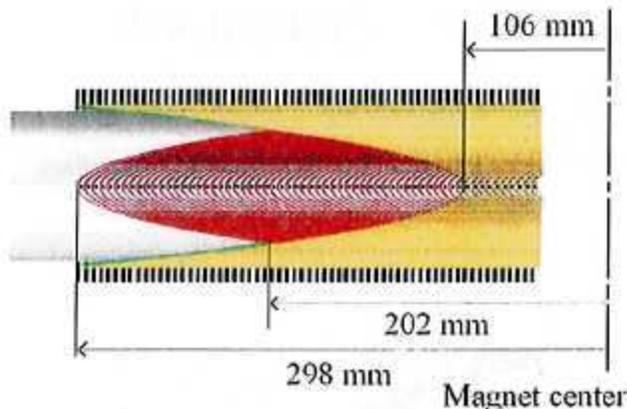
Fig. 2. Side view of the end region of the quadrupole magnet winding.
