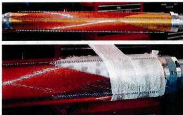
Fig. 4. Photos of the magnet before and during final glass wrapping.
