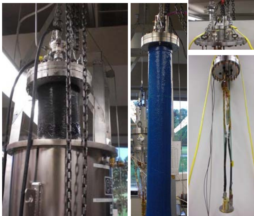
Figure 103. Photographs of the calorimeter used for ac loss measurements of superconducting coils.
