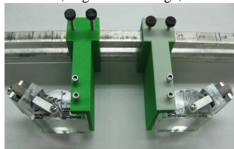
Figure 23. Transducer holder system showing the two transducers, the two wedges and the holding bar.
