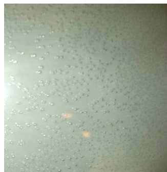
Figure 9. Photograph of sample after 120 °C bake test showing bubbles throughout the PVB interlayer in the glass.
