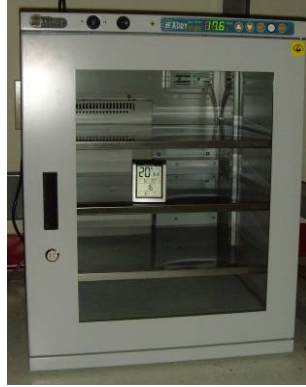
Figure 4. Controlled humidity storage for PVB interlayers at the RF lamination facility for maintaining humidity levels below 20%.
