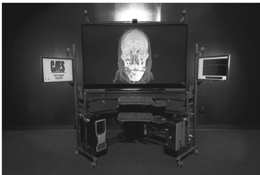
Fig. 2. The IQ-station, a mobile integrated immersive display system. This model uses two PCs, one for tracking and one for rendering.
