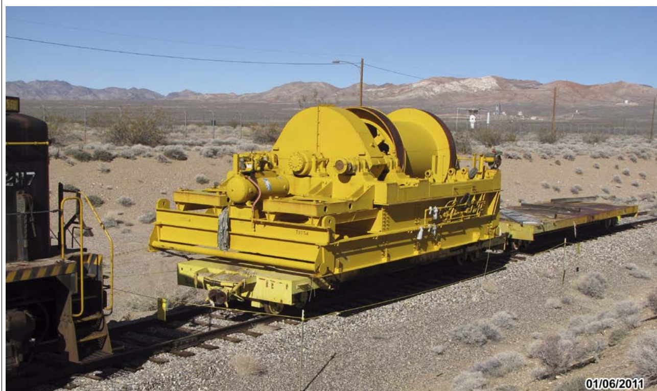
Figure 2-6 EMAD Compound Cable Spool and Flatcar
