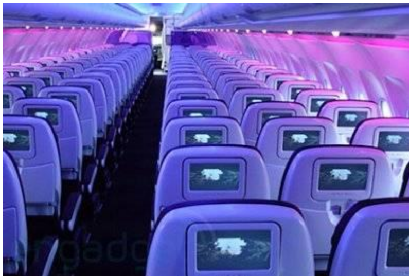
Figure 6: Illustration of typical in-flight entertainment (IFE) seat-back devices. The total IFE load on a 787-8 could reach 20 kW during all phases of flight. Note: Picture is not from a 787.
