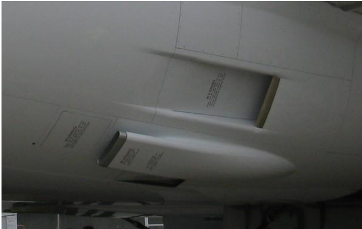
Figure 3: Ram-air inlet ducts on the 787 [16].
