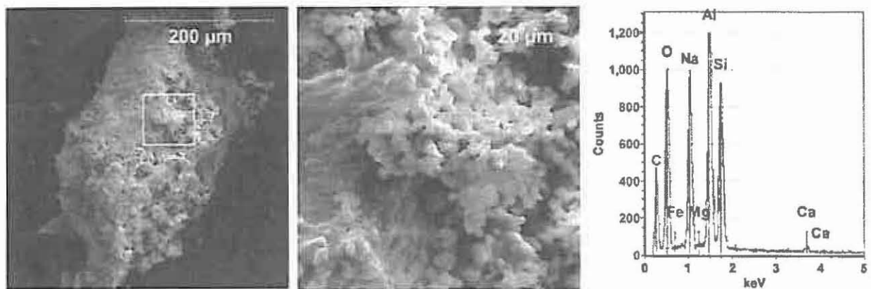
Fig. 4. Secondary electron image and energy dispersive X-ray spectrum of heavily coated garnet grain after three weeks at 80 °C.
