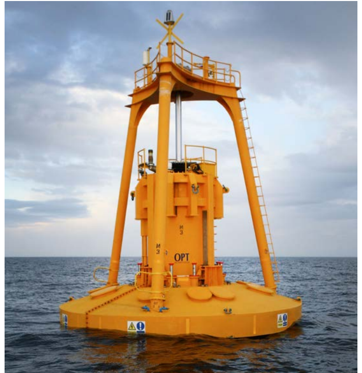
Ocean Power Technologies of Pennington's new 150-kilowatt PowerBuoy system captures the kinetic energy of waves to drive a generator that produces electricity. Photo from Ocean Power Technologies, NREL 22857
