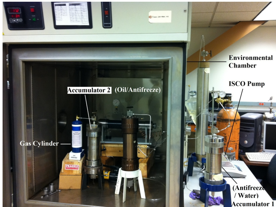
Fig. 5. Picture of the actual experimental setup for conducting CCE tests.
