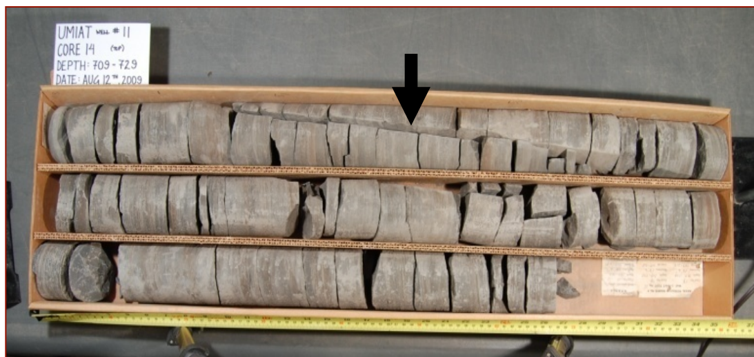
Figure 7: Fracture with an 82° dip in Umiat Well #11 , depth of 709 – 729’.
