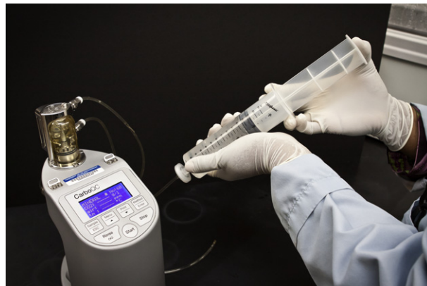
Fig. 1. Water sample being injected into the tested carbonation meter using a 140-mL syringe and an in-line 0.45-µm filter.
