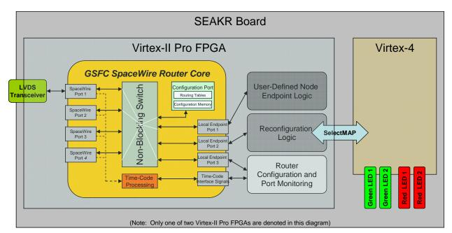
Figure 28. Configuration target (SEAKR) block diagram.
