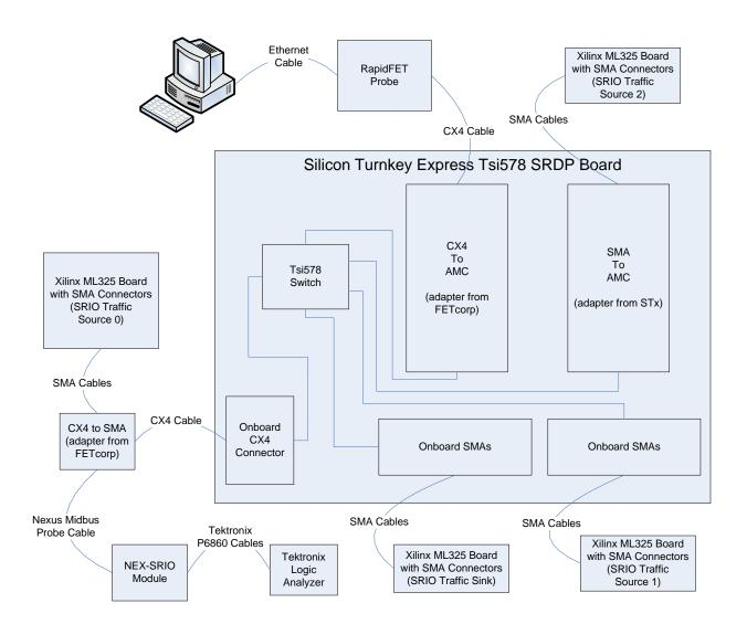
Figure 23. Debug and analysis system setup.
