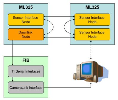
Figure 26. SpaceWire hardware demonstration layout.
