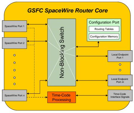
Figure 24. GSFC SpaceWire router IP core block diagram.
