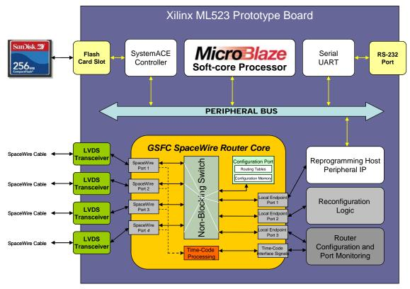
Figure 27. Configuration host (ML523) block diagram.
