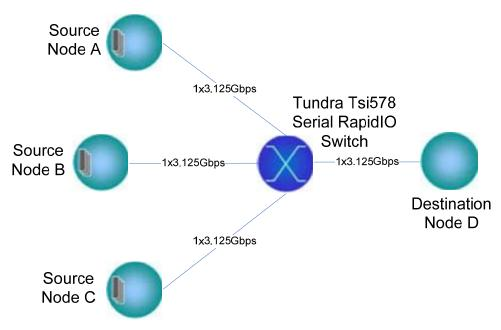
Figure 4. Test network topology.<sup>1</sup>
