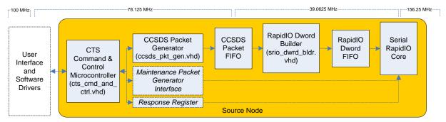
Figure 5. Block diagram of source node design.
