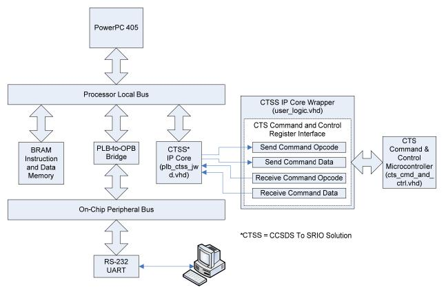
Figure 8. Software/hardware architecture.
