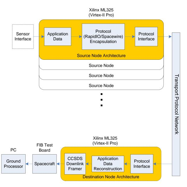
Figure 2. Detailed block diagram of hardware demonstration.
