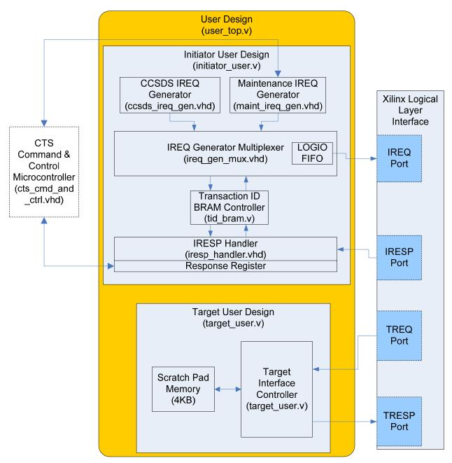
Figure 11. User design internal components.
