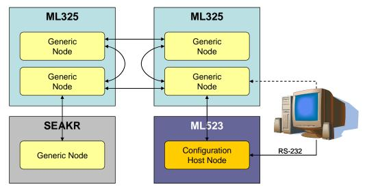
Figure 29. System block diagram for reconfiguration demonstration.
