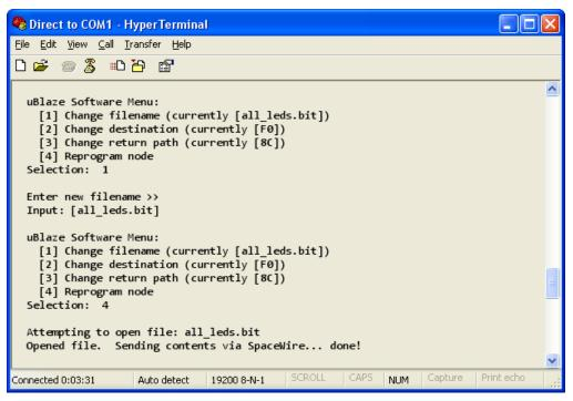
Figure 30. Remote configuration over SpaceWire control interface.
