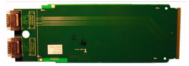
Figure 17. CX4-AMC Adapter Card (courtesy Fabric Embedded Tools Corporation [12]).
