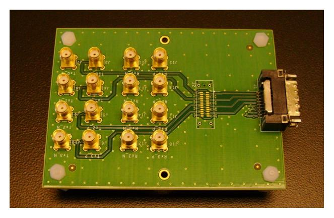
Figure 21. CX4-SMA adapter board (courtesy Fabric Embedded Tools Corporation [12]).
