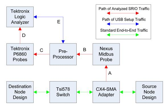
Figure 20. Nexus SRIO Protocol Analyzer connection topology (adapted from [14]).
