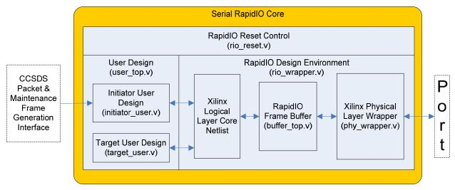
Figure 10. Block diagram of Serial RapidIO Core design.
