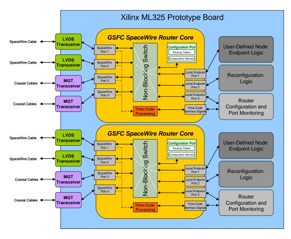
Figure 25. Two independent node instantiations on one ML325 board.
