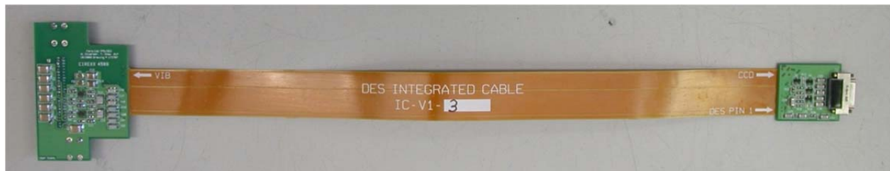
Figure 3. Semi-rigid Kapton cable. One end of the cable plugs into the Vacuum Interface Board and one end into the CCD pedestal package.
