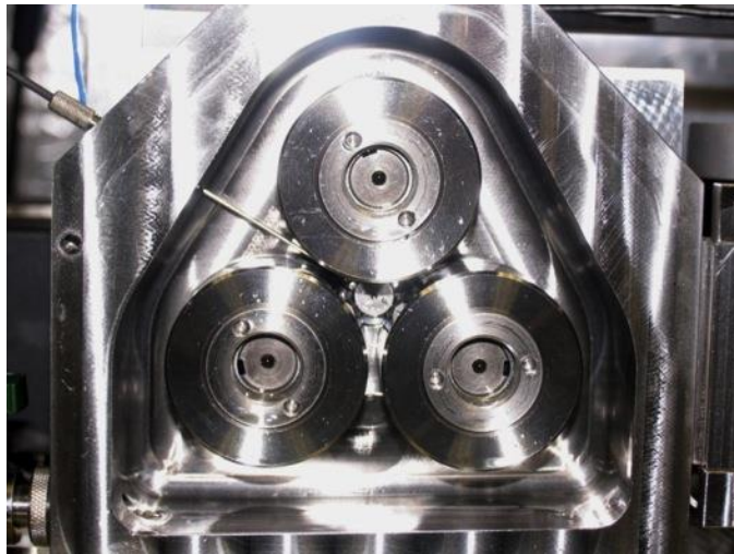
Figure 3. Cluster to rollers surrounding a smaller central test roller (chamber door open). The temperature probe enters the chamber from the upper left.
