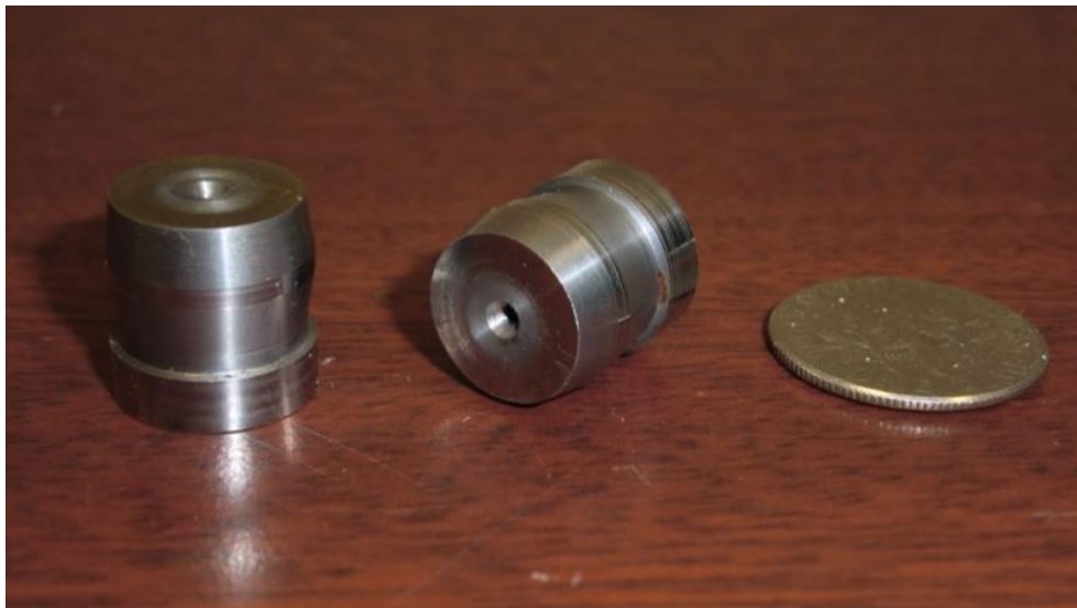
Figure 8. (a) Drawing of the test specimen, and (b) specimens after rough machining.
