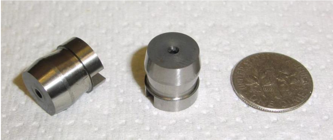
Figure 9. The test specimen (440XH) after final machining.
