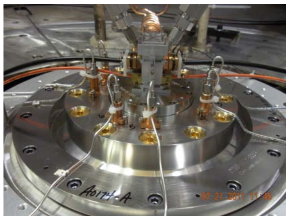
Figure 3.1. Image of the experimental setup at Z. Gas lines and the cold rod from the cryostat are visible in the image.
