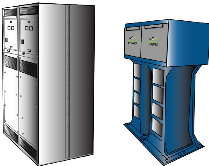
Lineage Power’s SMR System (right) compared with Conventional Ferro-based Rectifier (left)
