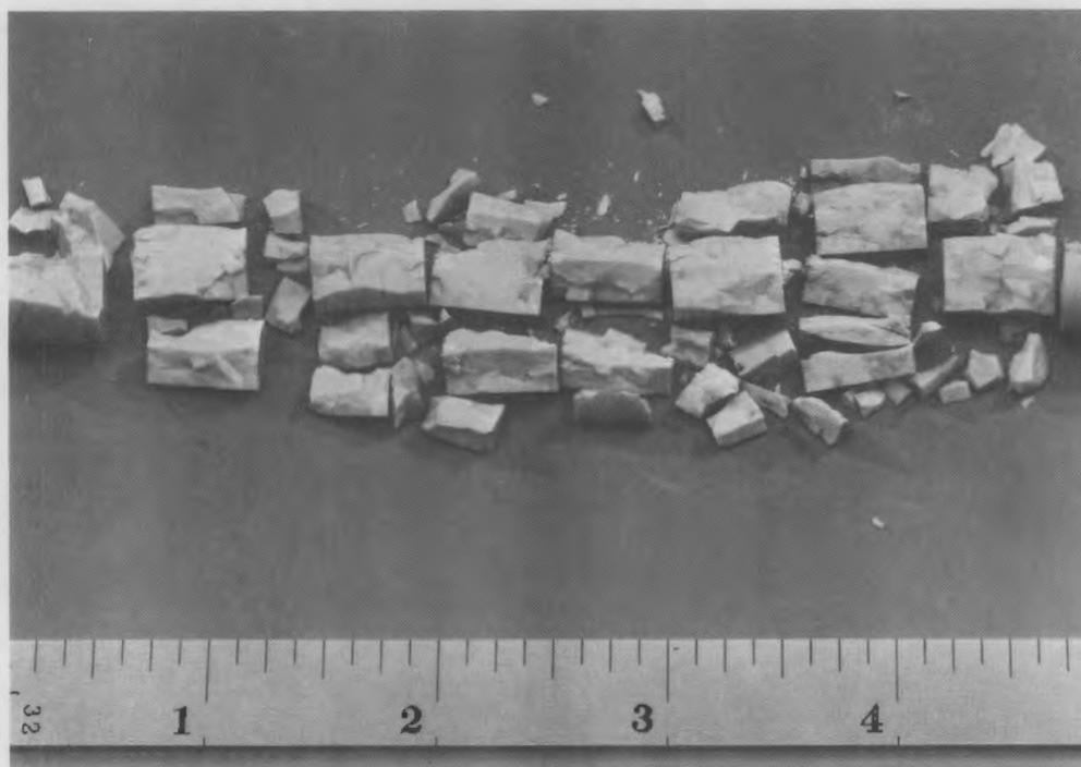
FIGURE 16d. Top of Rod 3 Disassembled Pellet Column
