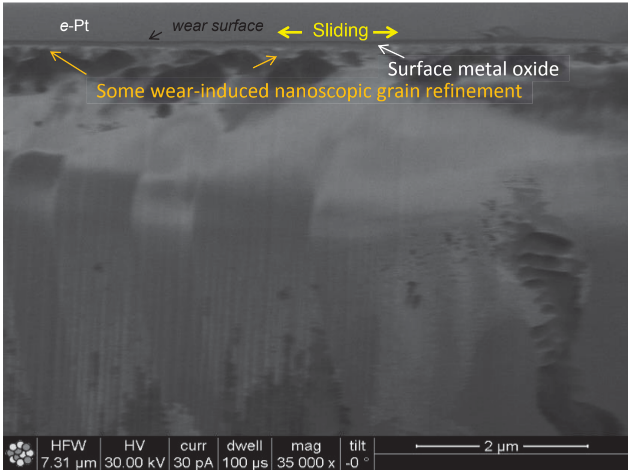
Figure 3.17. FIB-SEM image of AR+Aged A-286 alloy inside the wear track.
