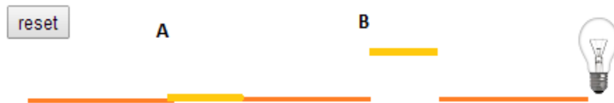
Figure 3.3 (a) AND gate with switch A closed
