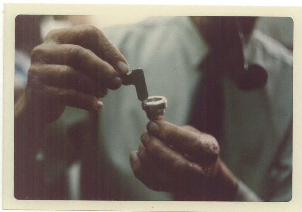
Fig. 10--Measuring the rim curvature
