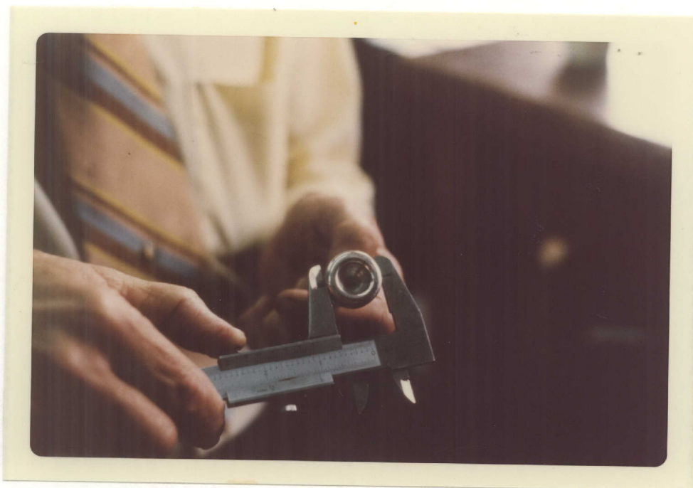
Fig. 9--Measuring the outer cup width
