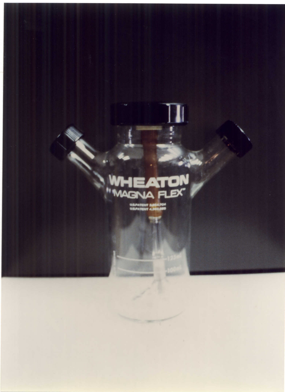
figure 1: A 125 ml Wheaton Magna-flex stirring flask.
