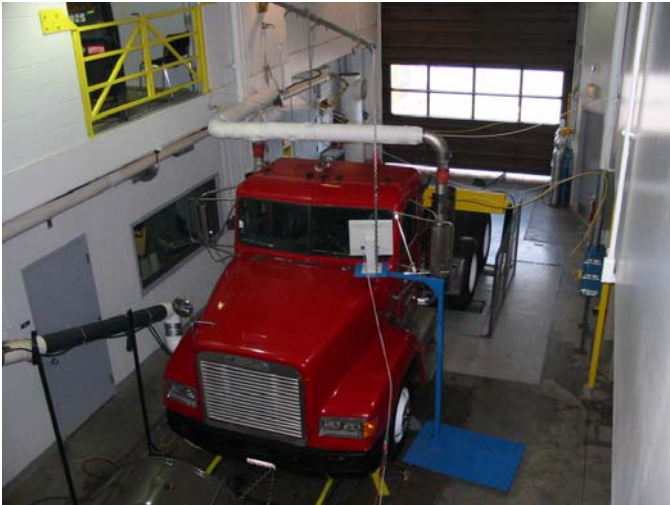
Figure 3. Test vehicle mounted on NREL ReFUEL chassis dynamometer.
