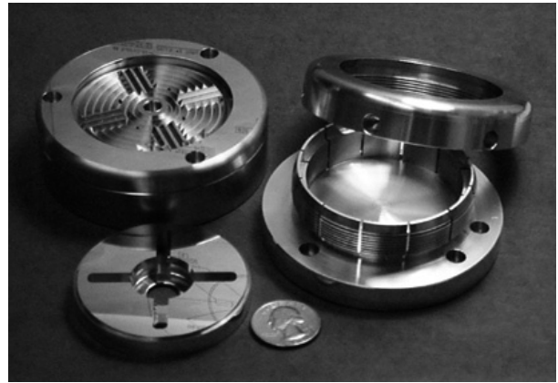
Figure 3: DDS-3 cell with diamond-turning fixtures.
