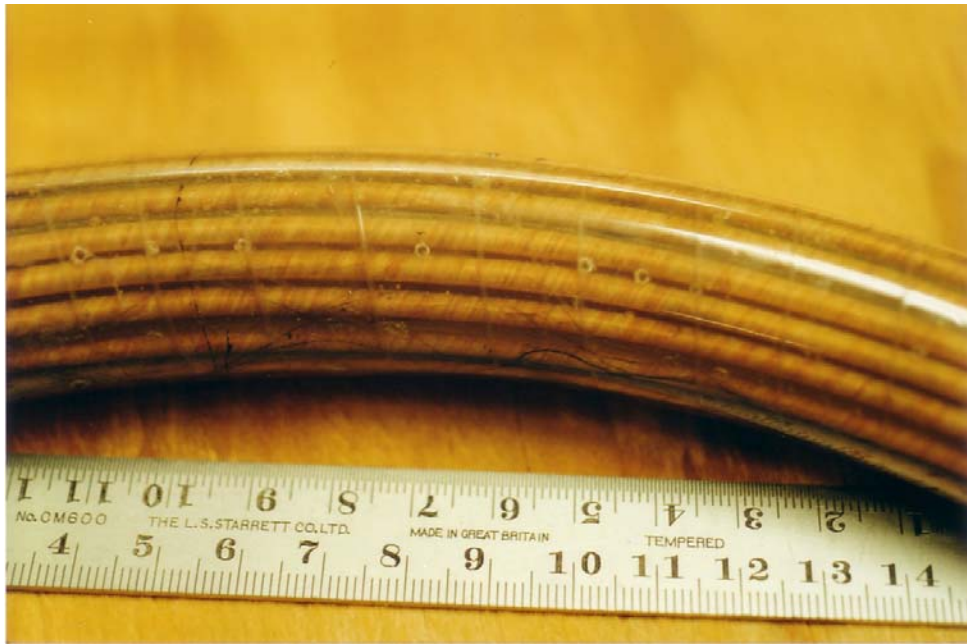
Figure 30. The FRC coil is wound as a hollow shell of 15 turns on the outside of a machined G10 form, reinforced outside with glass and carbon fiber windings, and vacuum-cast in epoxy. The scale is in cm.
