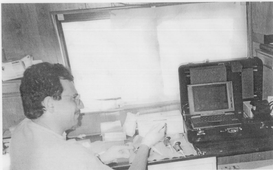
Figure 7. Photograph of the battery-powered, real-time PCR instrument in use at Dugway Proving Grounds in 1997. This instrument has control software that automatically calls a positive if DNA from the target organism is amplified during the thermal cycling. During this exercise, the typical time to detect was 20 minutes or less.
