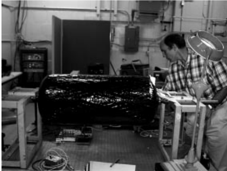
Figure 3. Lincoln Composite tank with optical fiber over-wrap.
