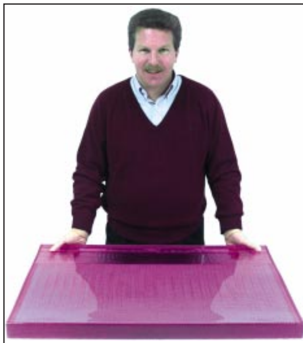
NIF Large-aperture phosphate laser glass blank as cut from a continuously melted glass strip.
