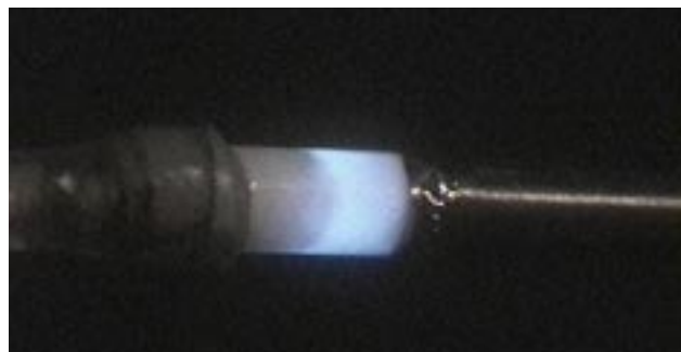
LLNL's x-ray catheter prototype, emitting a therapeutic x-ray dose (>6gy/minute).
