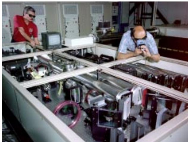
A zig-zag slab Nd:glass laser producing 60-J green output at <2\times diffraction limited at 3 Hz for Advanced Imaging Testbed experiments. This technology is also used for laser peening.
