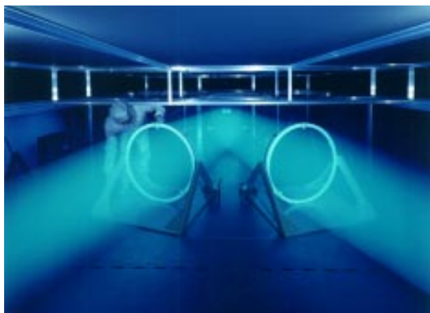
LLNL scientist inside the large-aperture diffractive optics production chamber, where the meter-scale diffraction gratings (used for compressing nanosecond spectrally chirped pulse to femtosecond duration) are produced.
