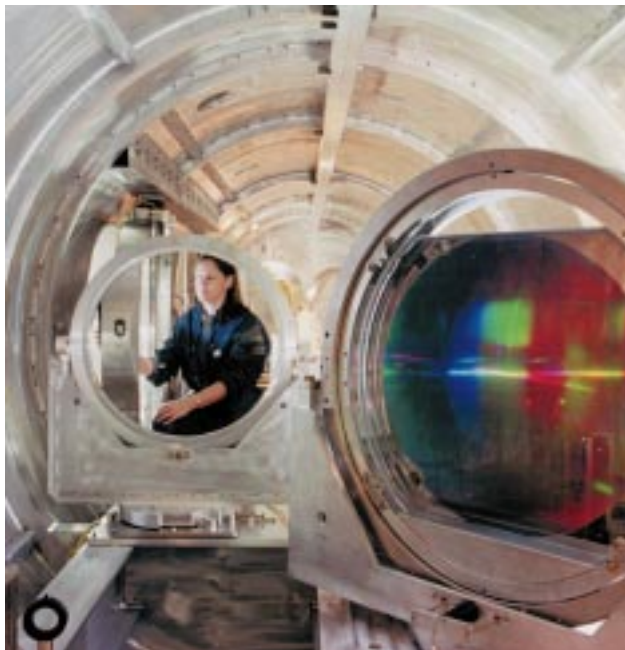
Scientist inside the Petawatt vacuum compression chamber at LLNL, which is used to compress a nanosecond-duration spectrally chirped pulse to less than one picosecond in duration. This temporal compression is performed by a pair of meter-scale gratings, one of which is seen on the right. The development of chirped-pulse-amplification laser technology has led to several industrially important spin-offs.
