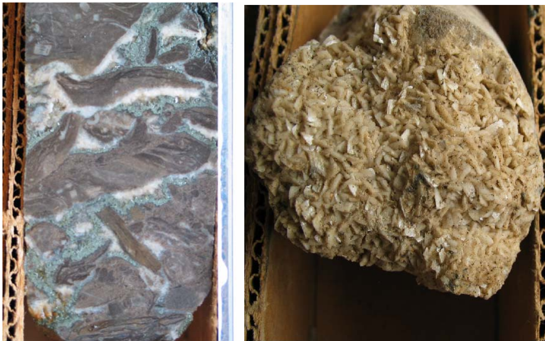
Figure 50. Left: Breccia with saddle dolomite (white) matrix dolomite (brown) and pyrite (gold) and right: saddle dolomite from cores in obviously fracture related dolomite areas in NW Ohio (sensu Wickstrom et al., 1992).
