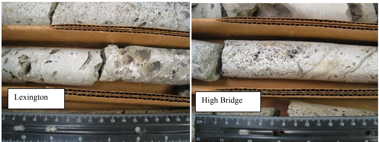
Figure 52. Porous dolomite from the Lexington (Trenton) and High Bridge (Black River) Groups in core JK-1 at Jephtha Knob in Kentucky.
