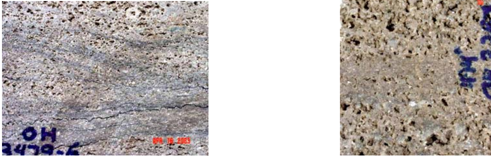
Figure 31. Dolograins from Trenton Group reservoirs in northwest Ohio. A. Dolograins with recognizable depositional texture. The rock consists of cross-bedded, coarse-grained crinoid-bryozoan grainstone interbedded with stylolitic dolomudstone/dolowackestone. These cyclic lithologies consist of shoaling-upward, grainstone-capped subtidal parasequences. Note the large crinoid allochem, which is mimetic planar-s to nonplanar-a (transitional) dolomite (also see Figure 32). The visible porosity consists mostly of small vugs, 0.5 to 4 mm in diameter, and molds. (OH 3479, Hancock Co., Palladin Enterprises, Anderson well, 1337.8 ft.). B. Interpreted dolograins without recognizable depositional texture. Dolomitization has obliterated all of this rock's primary and earlier diagenetic fabrics. The interpretation of this sample as a former grainstone is based on the presence of allochem ghosts, and both mimetic and non-mimetic replacement textures observed in thin section (Figure 33). (OH 3267, Auglaize Co. Meridian, Bousher #1 well, 1174 ft.).
