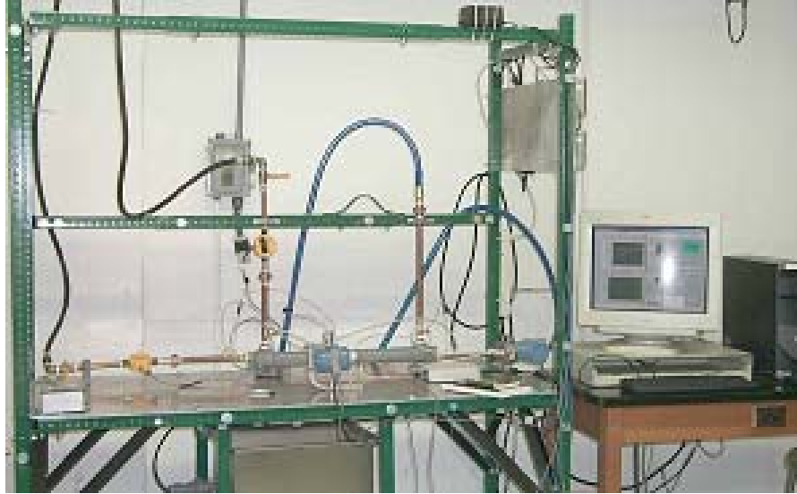
Figure 6.11. Photograph of the laboratory heat exchanger system.
