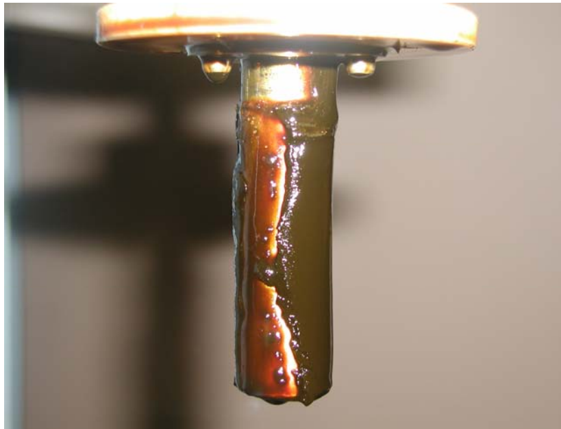
Figure 3.17 - Deposit for \Delta T=30^\circ F (Test 15)
