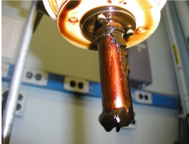
Figure 3.18 - Deposit for \Delta T=45^\circ\text{F} (Test 16)
