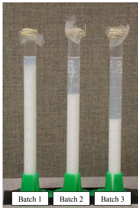
Figure 3-1: Sedimentation test results of spinel powders from Baikowski International after 106 days. The solid loading of each batch is 15.7 weight % and the solvent are 18.66 g of 2-propanol and 2.12 g of 1-methoxy-2-propanol. In Batch 1, 50 \mu L of fish oil and 0.2 g of PVP are added. In Batch 2, no dispersant is added. In batch 3, 50 \mu L of Darvan 811 is added. All batches are ball milled for 21.5 hours.
