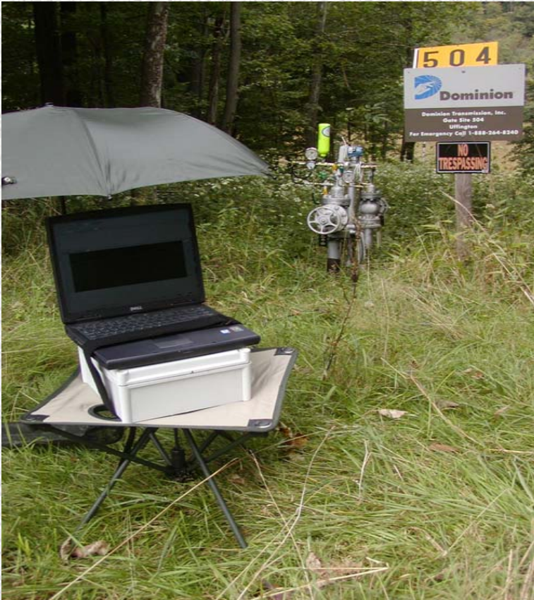
Figure 9 - PAMP and data acquisition unit installed on a natural gas transmission line in West Virginia. Computer, shielded cables and plumbing tree are clearly visible.
