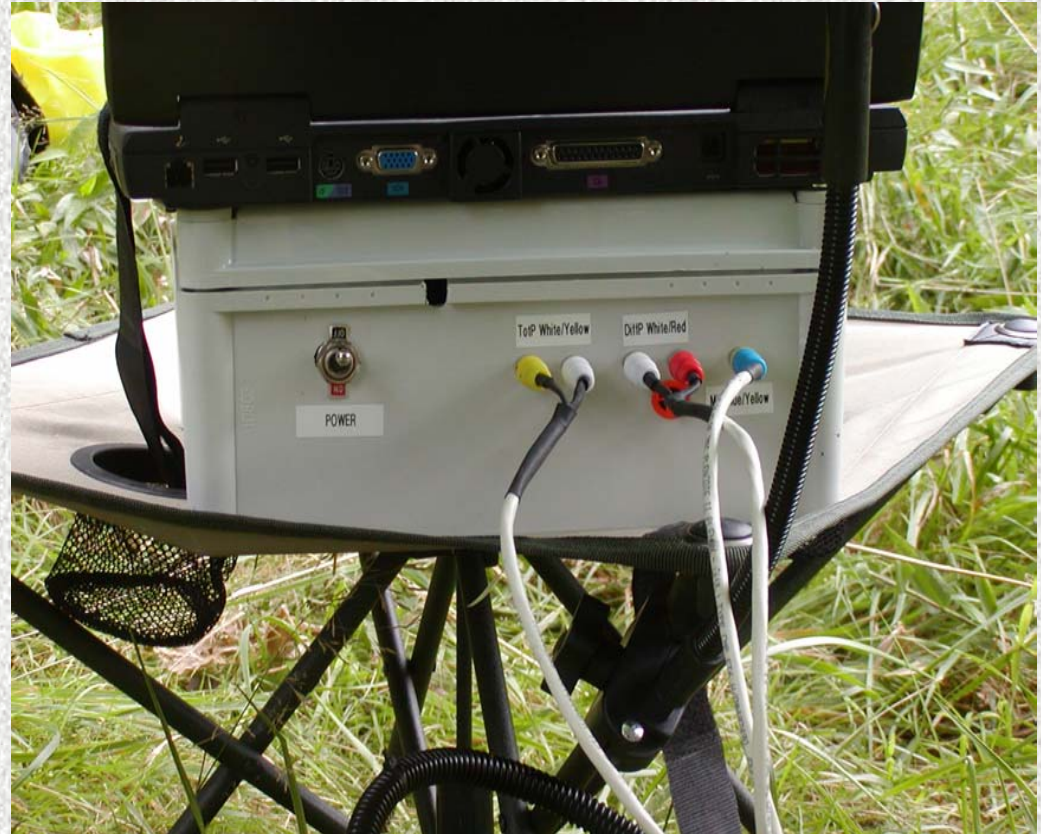
Figure 9 - PAMP and data acquisition unit installed on a natural gas transmission line in West Virginia. Computer, shielded cables and plumbing tree are clearly visible.
