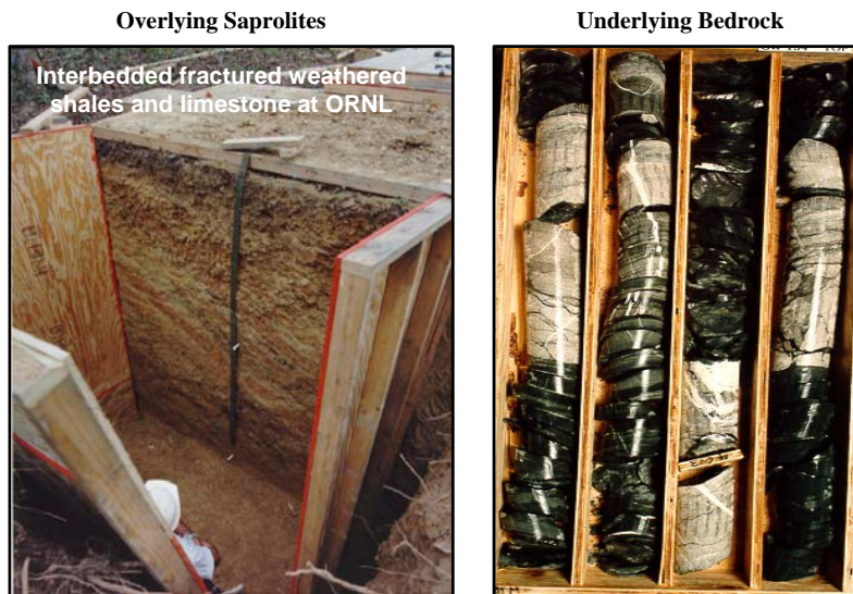
Figure 2: Typical subsurface media on the Oak Ridge Reservation consisting of interbedded shale – limestone sequences with characteristic dipping bedding planes.
