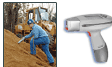
Figure 11: Field portable X-ray Fluorescence of quantifying metals on soil and sediments
