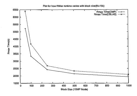
Figure 9.14  $R_{max}$  times for problem size 15000 with increasing block size. Using OpenMP
