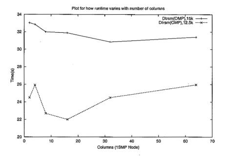
Figure 9.18 Dtrsm times for problem sizes 15k and 12.5k with block size 100. Using OpenMP
