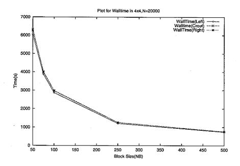
Figure 9.1 Runtimes (in seconds) for various block sizes, and varying the panel factorization. Problem size N=20000. Data from Table 9.1.
