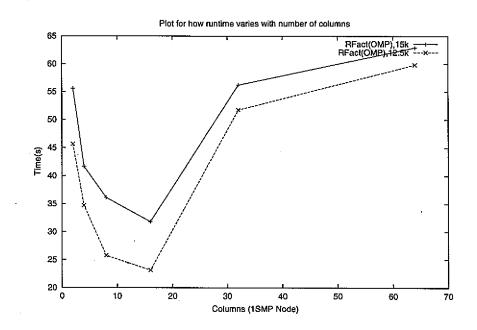
Figure 9.16 Factorization times for problem sizes 15k and 12.5k with block size 100. Using OpenMP
