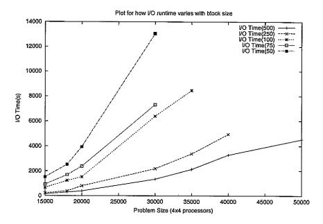
Figure 9.9 I/O Runtimes (in seconds) for different problem sizes with varying block sizes on a 4x4 processor grid. Buffer size is 2.
