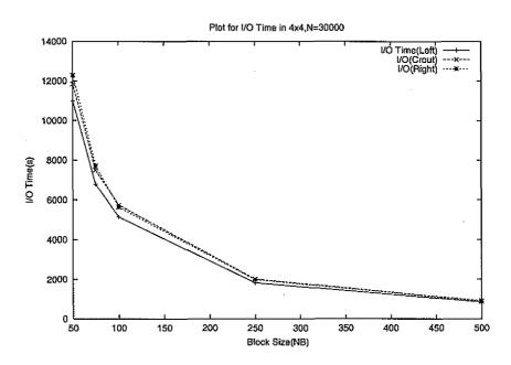
Figure 9.5 I/O Time(in seconds) for 4x4 processors, N=30000. Data from Table 9.2.
