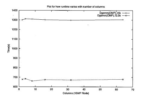
Figure 9.17 Dgemm times for problem sizes 15k and 12.5k with block size 100. Using OpenMP
