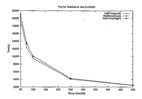
Figure 9.4 Runtime(in seconds) for 4x4 processors, N=30000. Data from Table 9.2.
