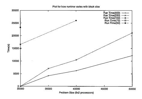
Figure 9.12 Runtimes(in seconds) for different problem sizes with varying block sizes on a 8x2 processor grid.Buffer size is 2.Communication is 1RingModified
