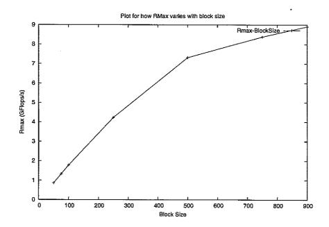
Figure 9.3 RMax values for 4x4 process node with varying block sizes. Problem size N=20000. Data from Table 9.1.
