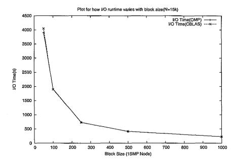
Figure 9.15 I/O times for problem size 15000 with increasing block size. Using OpenMP
