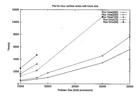
Figure 9.10 Runtimes (in seconds) for different problem sizes with varying block sizes on a 2x8 processor grid.Buffer size is 2. Communication is 1Ring Modified
