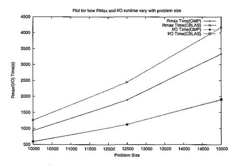
Figure 9.13 Plot for varying problem size, with fixed block size of 100. Using OpenMP
