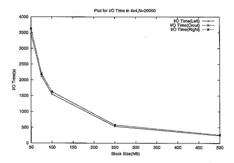
Figure 9.2 I/O Times (in seconds) for various block sizes, and varying the panel factorization. Problem size N=20000. Data from Table 9.1.
