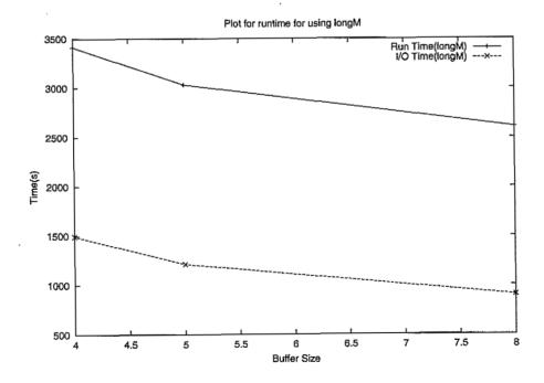
Figure 9.7 Runtime(in seconds) for problem size N=50000, running on 8x8 grid with block size 500 versus the buffer size. The broadcast type is Long Modified
