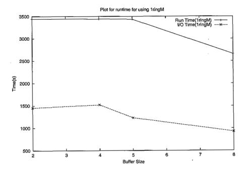
Figure 9.6 Runtime(in seconds) for problem size N=50000, running on 8x8 grid with block size 500 versus the buffer size. The broadcast type is 1Ring Modified
