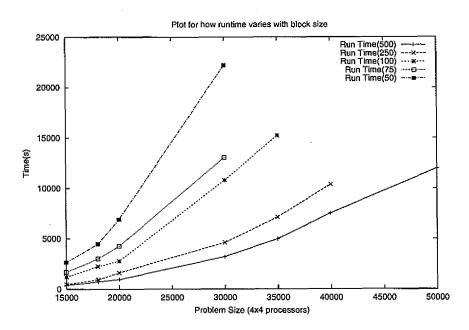
Figure 9.8 Runtimes (in seconds) for different problem sizes with varying block sizes on a 4x4 processor grid. Buffer size is 2.
