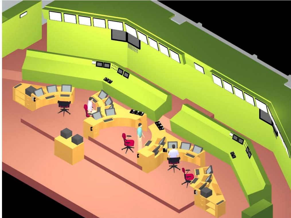
Figure 2-10 3D View of the Concept Shown in the Layout of Figure 2-9 (Benchboard and Vertical Panel Controls and Indicators Not Shown)
