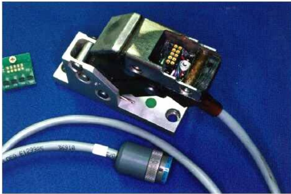
Figure 21. A sensor head with replaceable sensor circuit.
