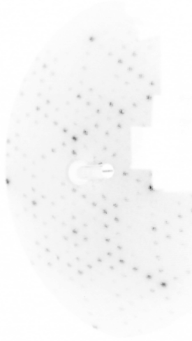
Figure 2.10: LEED image of clean, reconstructed Si(111)7 \times 7 surface.
