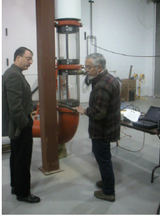
Figure 2. Transparent Coal and Air Test Section
