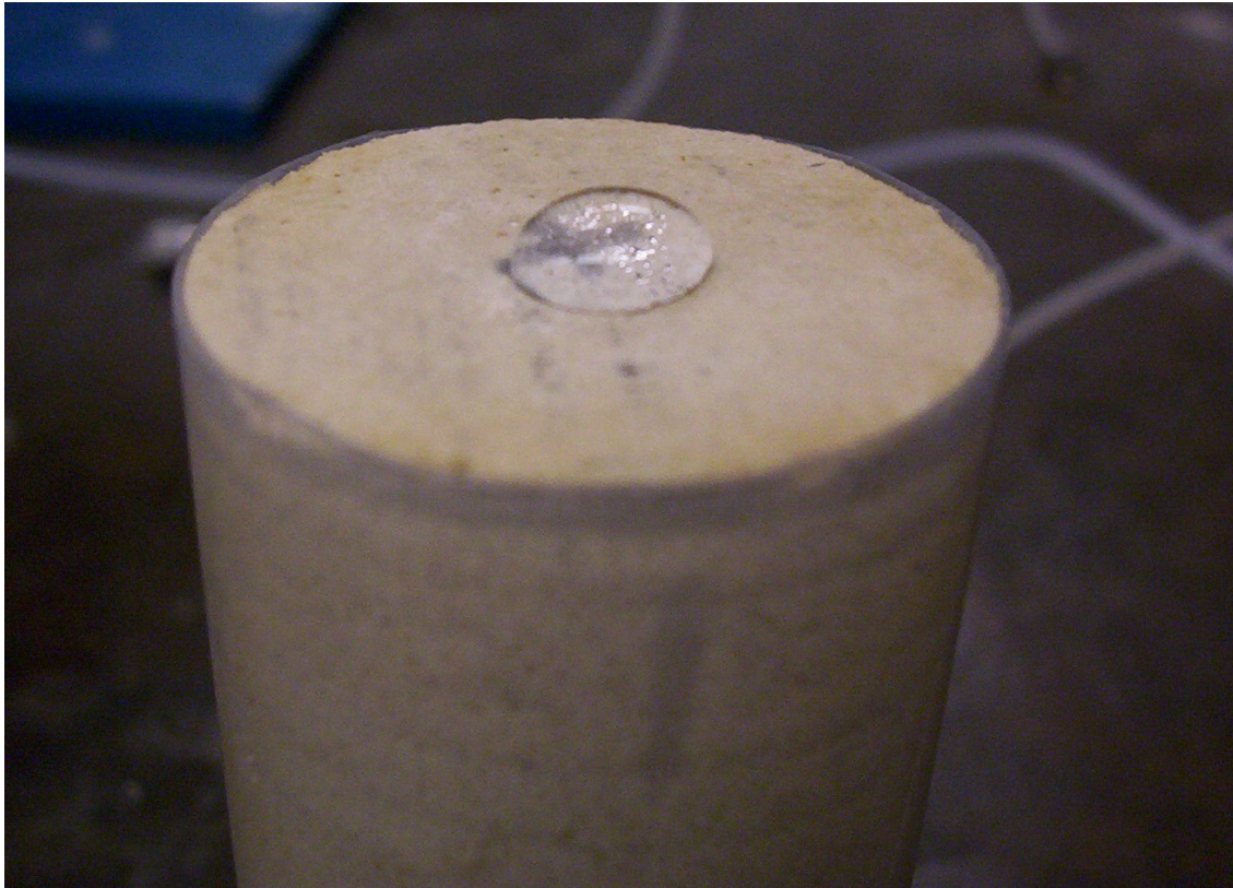
Figure 1: Photograph of the core after treatment with surfactant F, indicating change in wettability of the surface. The drop of brine does not imbibe spontaneously into the carbonate rock.
