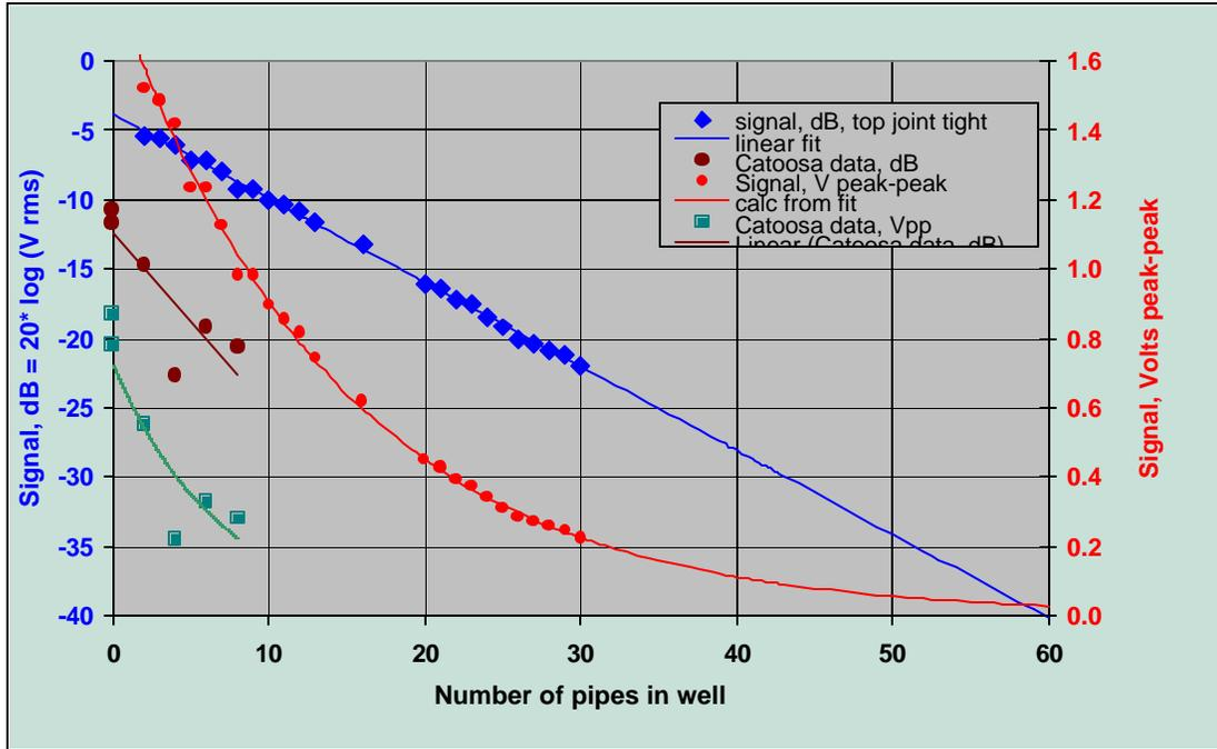
**Figure 2.** Transmission line strength as a function of number of pipes
