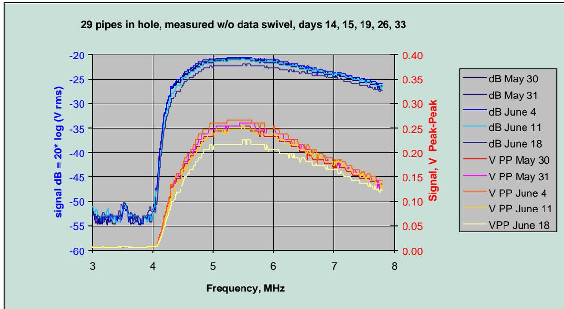
**Figure 3.** Transmission line strength as a function of time in well
