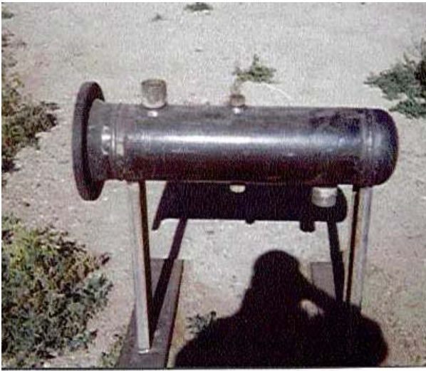
Prototype "Filter Canister" From Steel Pipe
